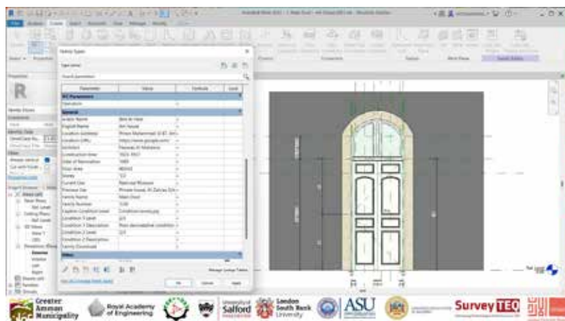
Fig.3. The final Revit model includes the option to alter dimensions and characteristics of objects. Image courtesy of V. Cotella [7].
