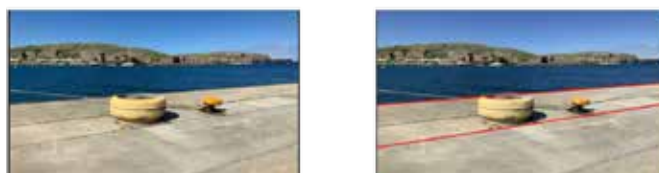
Fig. 2. Original image and Result of Visual Monitoring Points Extraction (red boundary lines of the quay).
